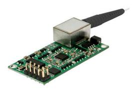
Agiltron offers Fiber Optic MEMS Tunable Filters with central wavelengths of 1060nm, 1310nm, 1550nm, and 2000nm. It is tunable continuously over a spectral range of up to 80nm at a speed of about 80ms. The wavelength tuning is actuated by driving a rotating MEMS mirror that is optically coupled with a grating and a dual fiber collimator. It is conveniently controlled with user-friendly GUI and control interfaces of USB or RS232 and I2C.
